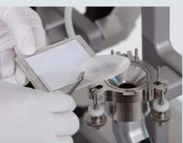
The suction extraction directly via the filter unit is suitable for small surfaces with low particle load, for example in the process environment on workpiece carriers or on circuit boards. Particle collection is fast, minimizing process interruptions.
