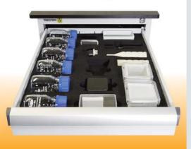
The extraction and analysis equipment is directly accessible in special drawers below the work surface and the extraction unit. Precisely fitting drawer inserts ensure cleanliness and tidiness in the drawers.
