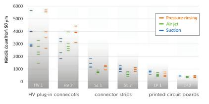
production batches and then tested and analyzed using these three extraction processes. The study focused on the total number of particles in several individual analyses and the breadth of their dispersion among them.
