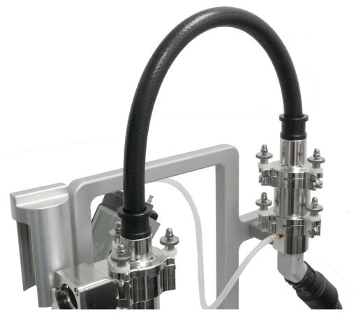
Interconnecting cyclone unit and filter unit
