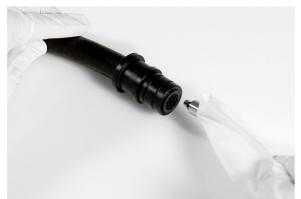
Inserting the alcohol-soaked cleaning cloth
