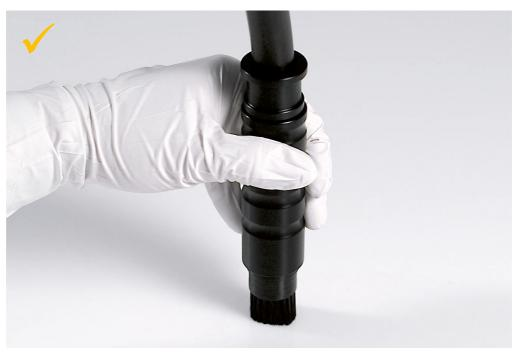
Applying the brush nozzle correctly
