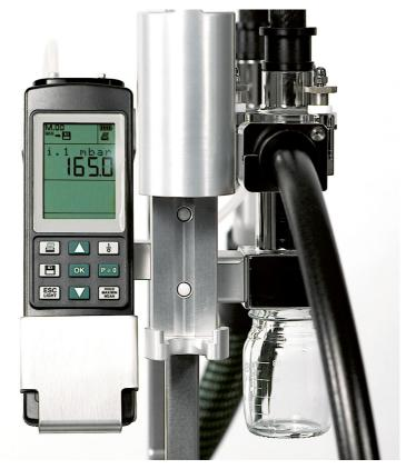
The differential pressure measuring device
