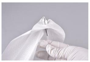
Cleaning wire with attached alcohol-soaked cleaning cloth
