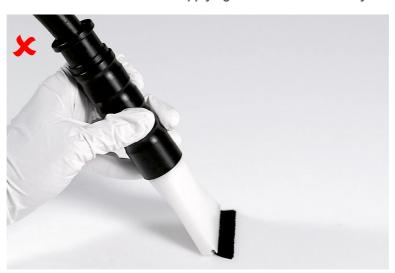
Applying the flat nozzle incorrectly
