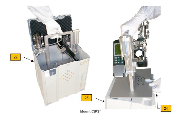
⇒ Lift particle suction extraction system out of the transport box (22) and attach it to the equipment case (23). Close locking mechanism (24).
