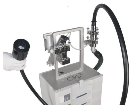
Determining the blank value, suction with prefilter
