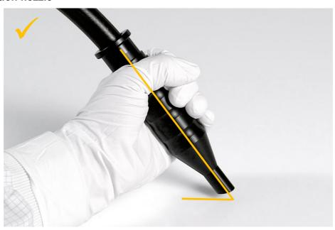
Correct distance and angle to hold the suction nozzle
